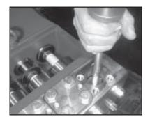
2. Take out complete valve assemblies (51 and 52) using either tool (part #07662) or stud bolt.
